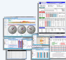
2004: SoftMaid Software Displays Pump Station Abnormal Behaviors and Generates Pump Efficiency Reports
