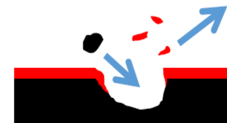
4. Further erosion maintains contact between base material and erosive fluid
